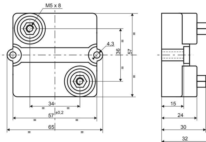
"Connection and mounting screws are supplied with the resistor
